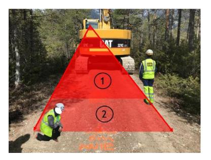
1./ Lack of visibility from the excavator when standing 2./ Lack of visibility from the excavator when kneeling.
