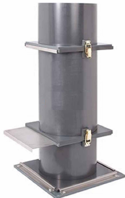
FIGURE A.6 ARRANGEMENT FOR STATIC SEGREGATION TEST IN ACCORDANCE WITH ASTM C1610
